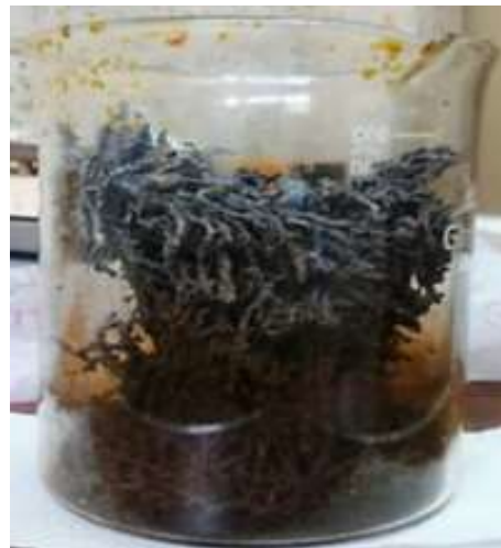
Fig. (3) Magnetite NPs final product prepared by sol-gel auto combustion
