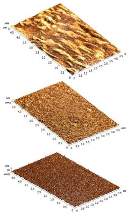
Fig. (2) 3D AFM images of MgO films at various concentrations of doping with TiO 2 (a) pure, (b) 3%, and (c) 5%
