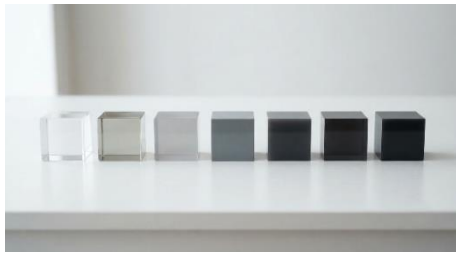
Fig. (1) A photograph of the nanocomposite sample fabricated in this work with different weights of \text{Co}_3\text{O}_4 NPs in the transparent resin host (from left to right: 0%, 2%, 6%, 10%, 15%, and 20%)
