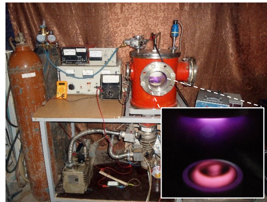
Fig. (2) DC sputtering system used in this work as the glow discharge plasma is seen inside the chamber
